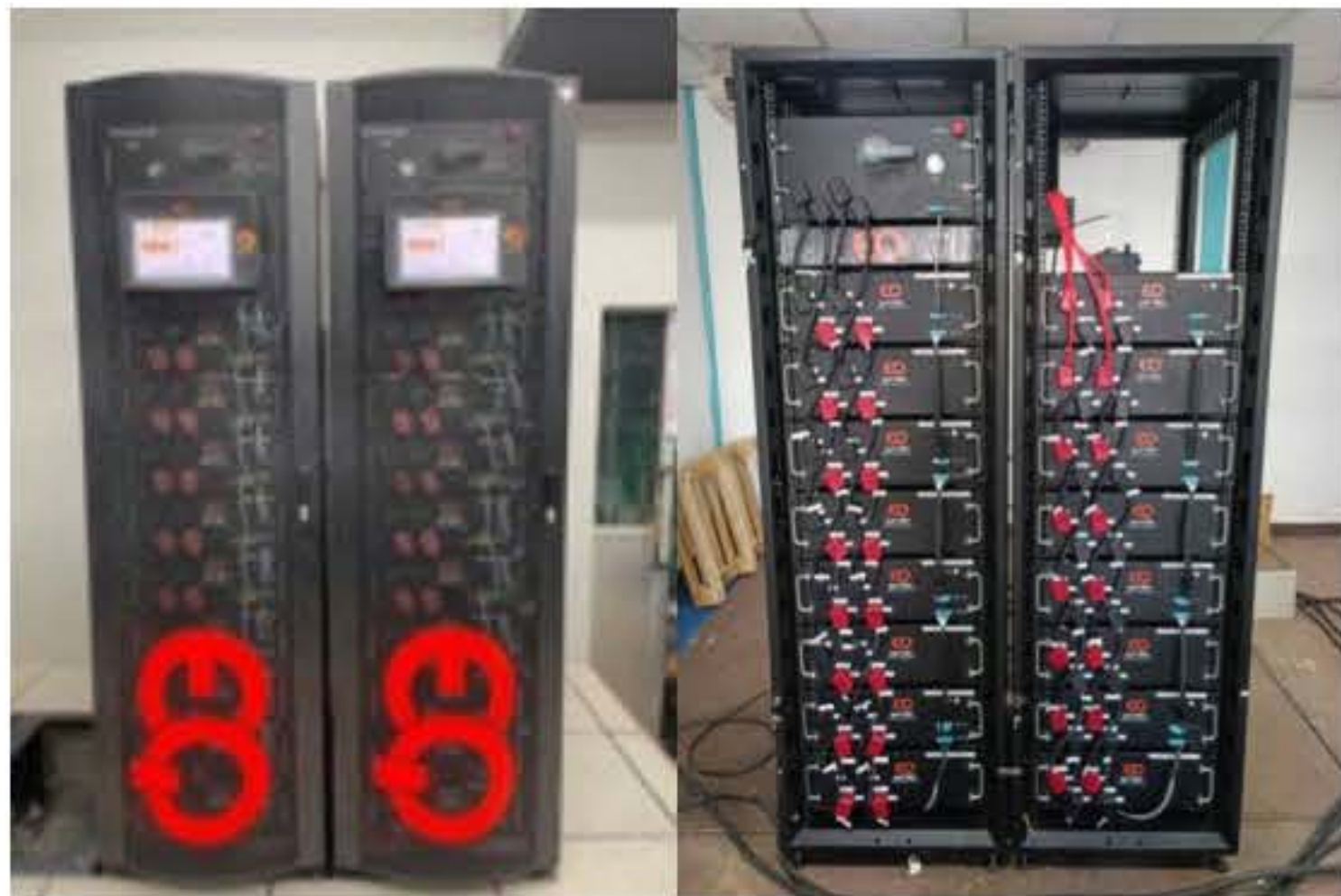
Figure 3. Prototype of a 100 kWh LiFePo4 battery with monitoring system.
