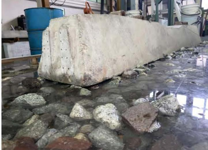
Figure 2 Experimental setup and flooding simulation of the ballast layer
