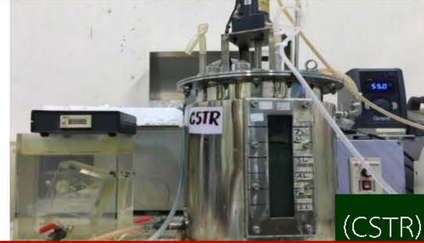
Acidogenic anaerobic dark fermentation 6 L working volume in CSTR
