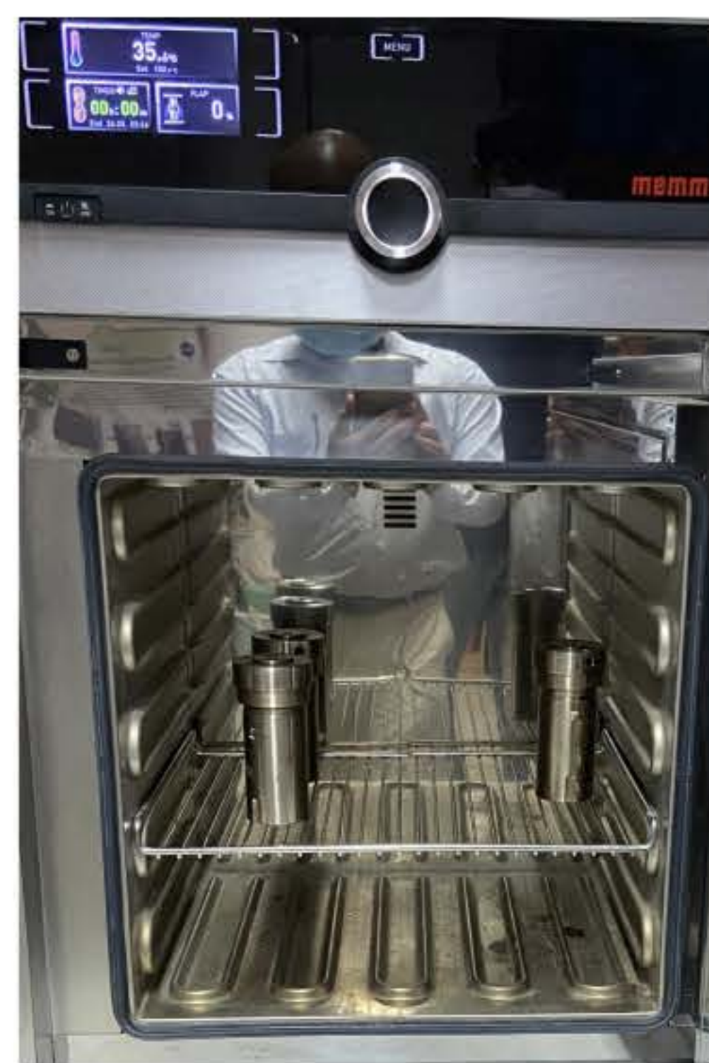
Figure 2. Hydrothermal synthesis of CQDs using a stainless-steel autoclave with a Teflon lining.
