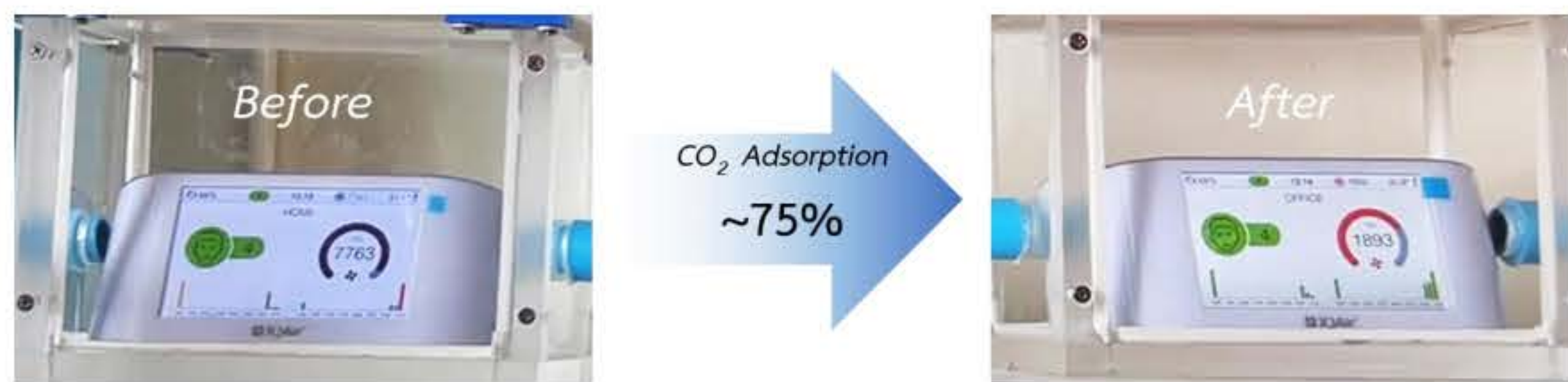
Figure 7. The result of CO 2 adsorption system with an NR-foam filter.
