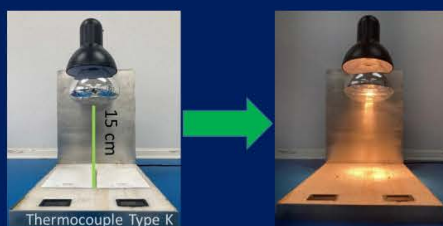
Fig.4 Schematic representation of the apparatus developed for exposure to IR radiation (ASTM E 903) .
