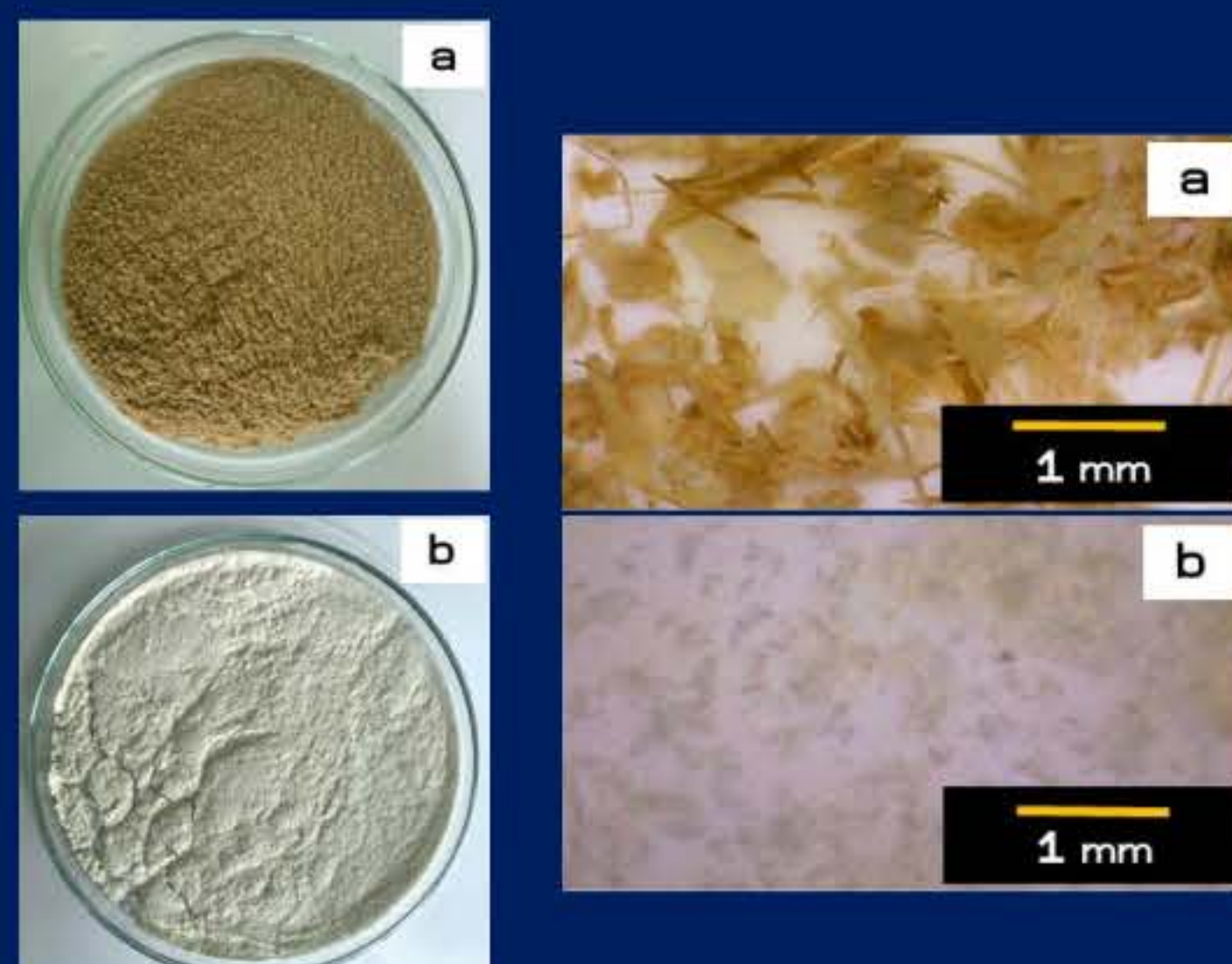
Fig. 1 natural bamboo (a) and (b) natural bamboo after synthesis and grinding with ball mill 2 hrs.
