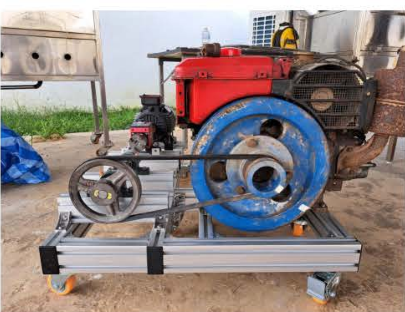
Figure. 2. Generator connected with IC-engine setting up
